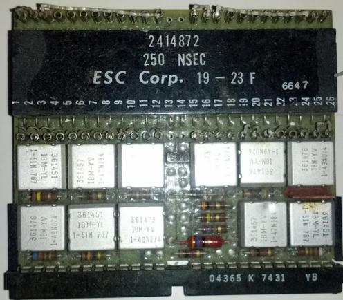
Delay line selectable in 250 ns increments
